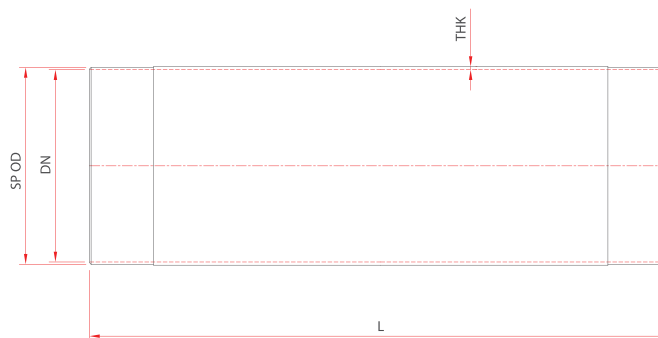
UNDER GROUND PIPE
